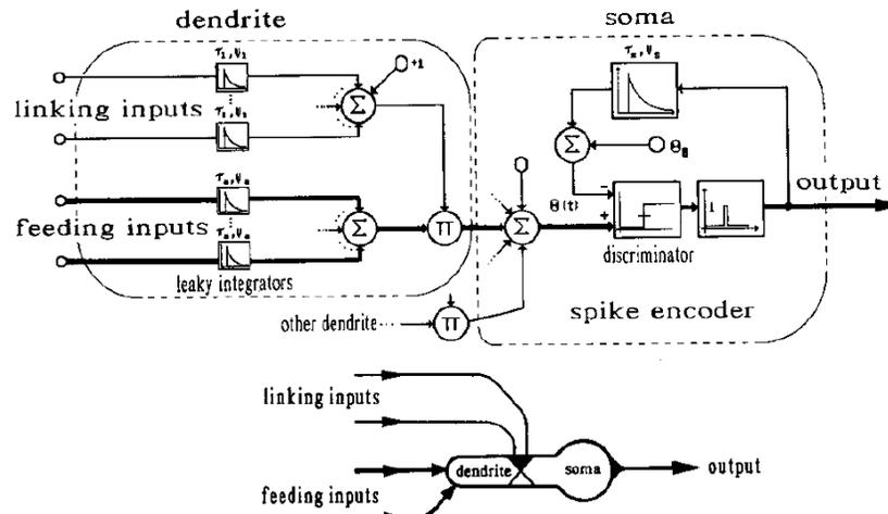
Figure 1.5. Basic Eckhorn neural unit (ENU) having two components (dendrite & soma). Inset shows internal workings in the components (adopted from [Eckhorn et al. 1990]).
