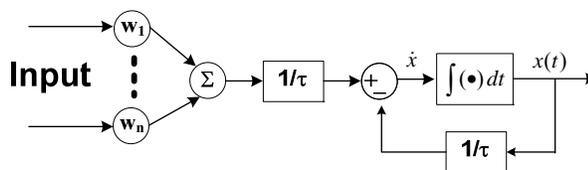
Figure 1.7. Block diagram of the leaky-integrator (LI). Feed-forward gain ( $1/\tau$ ) is used to make the transfer function have unity gain for step function inputs. This implementation is shown in equations (13) and (14).
