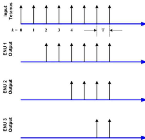
Figure 1.14. Illustration adopted from [Wells 2010, Ch.9] showing a simple ENU high-pass firing chain for a network consisting of three one-dimensional layers of neurons. The neural outputs from the end receiving stimulus to the third neural layer end demonstrate evanescent wave-like packets.
