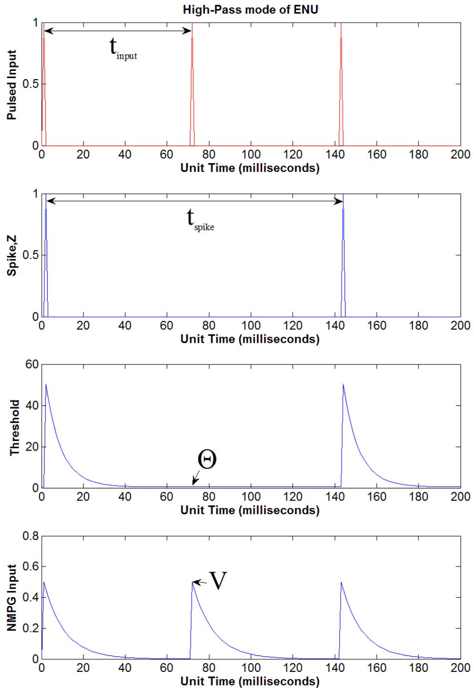
Figure 1.9. Snapshot of Figure 1.8b (High-Pass mode) demonstrating that the soma input ( $V$ , arrow of bottom plot) triggered by the second input (red, top plot) does not succeed in causing a spike because  $V < \Theta$ . Thus the inter-spike interval ( $t_{spike}$ ) is wider than inter-input interval ( $t_{input}$ ). That is, ENU at high-pass mode behaves like a high-pass filter as it filters out inputs with low rates.
